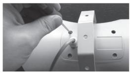
Remove the four screws from the top of the MPBD20-G
